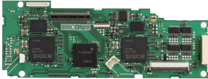
Dual "DIGIC III" processors for enhanced speed and image quality
